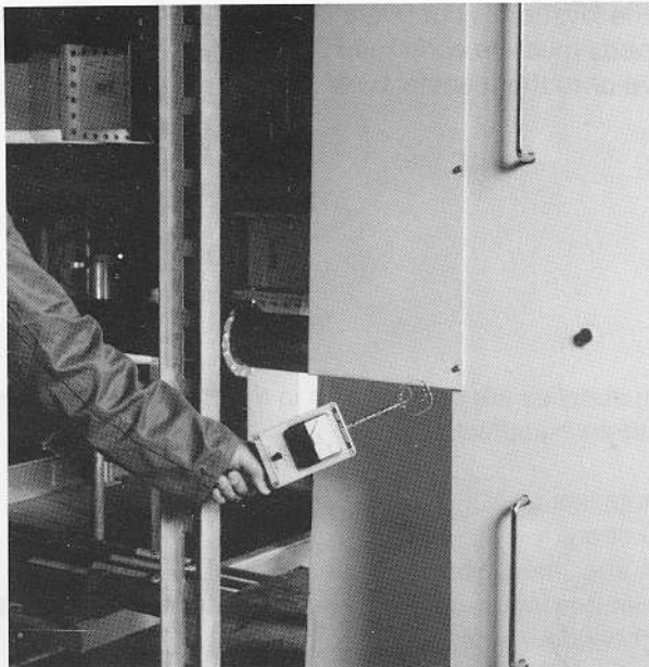
Fig. 57. Checking for RF Radiation Leakage
