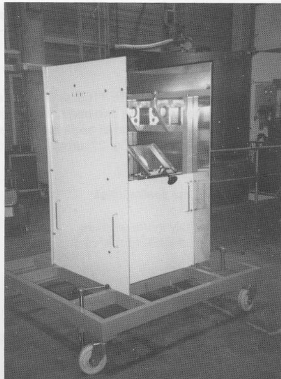
Fig. 19. Trolley (TE 1167) with Factory-Fitted Lead Shielding Plates (view from rear)
