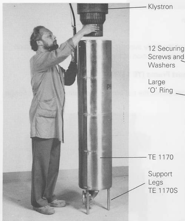
Fig. 17. Preparing to Lower the Klystron into its Collector Water Cooling Jacket TE 1170
